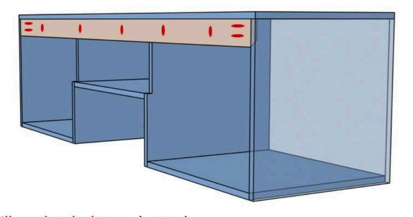
Drill pocket holes and attach top of French cleat with 1-1/4" pocket screws.
